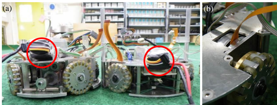
Fig. 10 (a) Lower height of new robot (right one; red circle shows the battery, left one is previous model) and (b) top of the motor for driving wheel.
